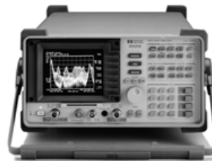
Spectrum analyzer measuring noise figure
