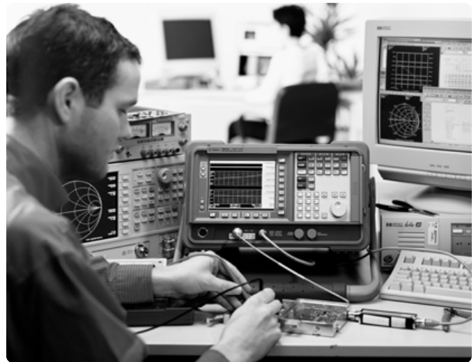
NFA simplifies noise figure measurements
